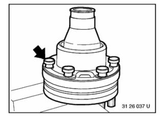
Mount new end cover and boot on propeller shaft or on constant-velocity joint.
