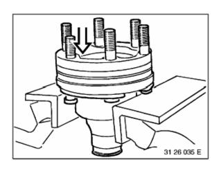
Drive out cheese-head bolts using a plastic hammer. Remove washers.
