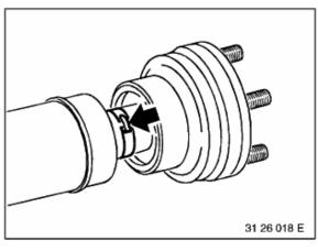
Pull boot onto propeller shaft.
